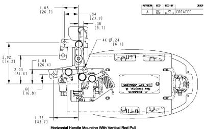
Horizontal Handle Mounting With Vertical Rod Pull
