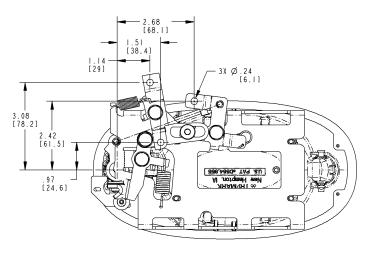
Horizontal Handle Mounting With Horizontal Rod Pull
